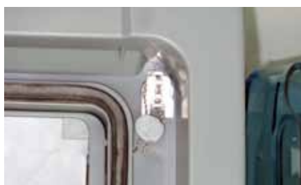
Sealing the screws on the front panel
